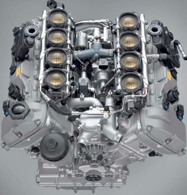
Individual throttle bodies for each cylinder help the new M3 4.0-L V8 engine produce 309 kW (414 hp) at 8300 rpm.
