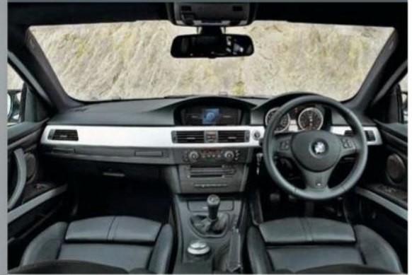
The steering wheel of the M3 provides an MDrive button for EDC (electronic damper control) and enhanced DSC+ (dynamic stability control) settings.
